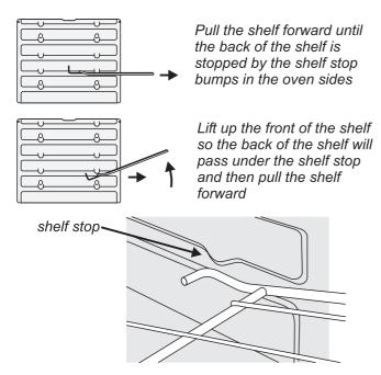
To refit the shelf, line up the shelf with a groove in the oven side and push the shelf back until the ends hit the shelf stop. Lift up the front so the shelf ends clear the shelf stops, and then lower the front so that the shelf is level and push it fully back.
